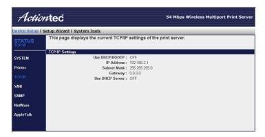
The screen displays the state of the Print Server's DHCP/BOOTP and DHCP Server connection, as well as its IP, subnet mask, and gateway addresses.
